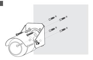
Installing using Wall Mount
