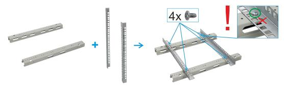
**Note** - the distances between the RACK profiles can be adjusted stepwise, front to back, according to the diagram below.
