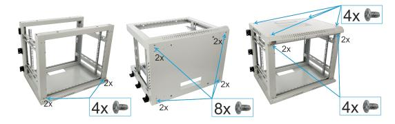
Connect the wall panel with the front part of the RACK cabinet. Screw the hinges to the wall panel. Install the cover plates at the bottom of the cabinet.
