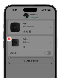
When Outlet [type F] malfunction is detected, the Ajax app displays a malfunction counter on the device icon. All malfunctions are indicated in the outlet's states. Fields with malfunctions will be highlighted in red.
