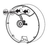
8-1 • Installing network/power cables
