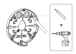
Directly installing on wall/ceiling
