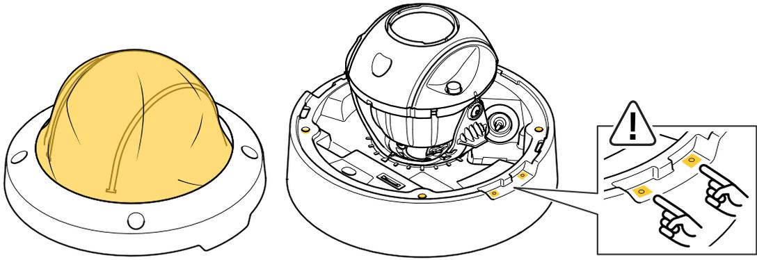
4. Mask the four screw holes. For AXIS Q3556-LVE and AXIS Q3558-LVE, mask the acoustic sensors.
