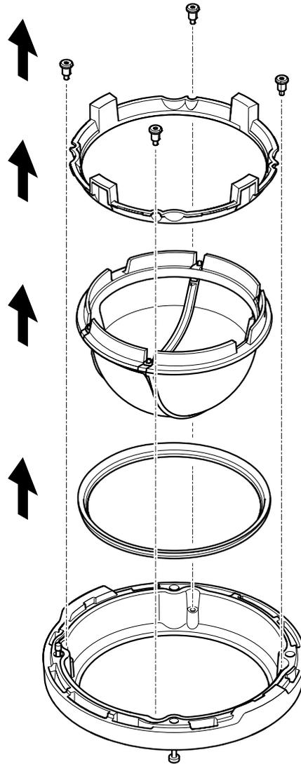
2. Remove the four screws, holder dome, dome and gasket dome.
