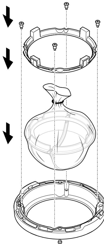
3. Reassemble the dome into the cover top.
