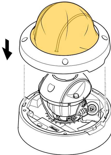
5. Remove the screws from the cover top. Put the cover top back on the camera.
