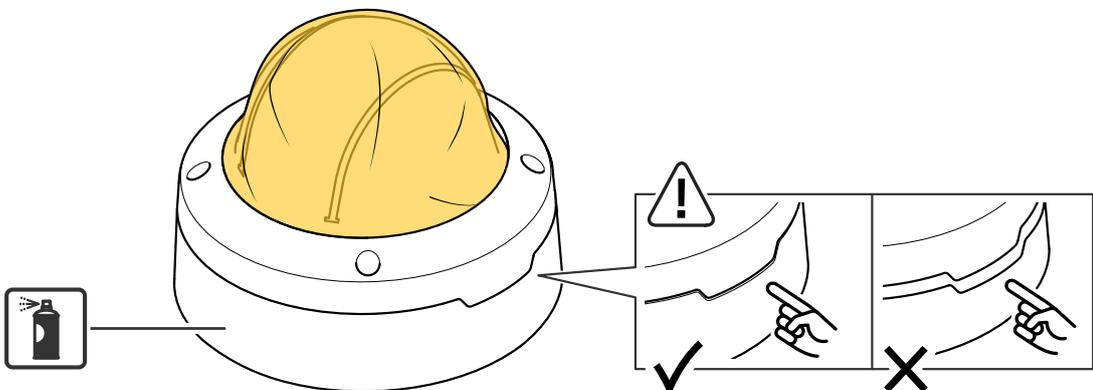
6. Apply a thin and even layer of spray paint according to the instructions of the paint manufacturer.
