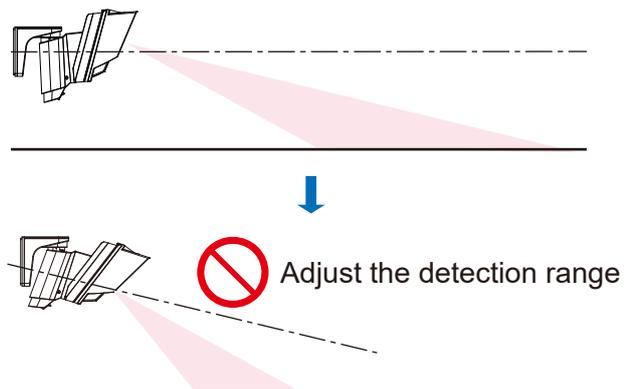
**2** Adjust the camera angle to view the detection area
