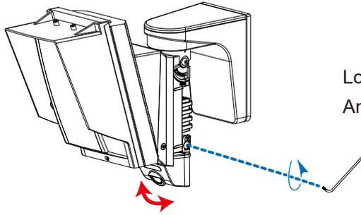
Loosen screws to adjust camera angle
