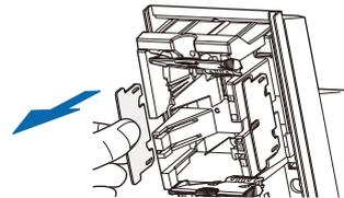
**2** Insert the plate into the position determined by the required masking distance until it clicks, see table below.
