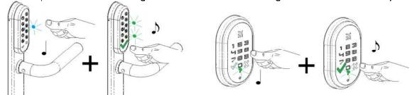
3. When all user and shadow cards are added, approach the programming card and the process ends. If this is not done, the device waits a few seconds finishing the process itself.
