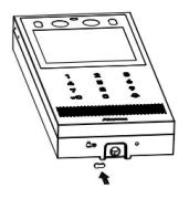
Place the silicone plug into the bottom of the device.
