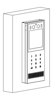
After pushing the device down into the bracket, you will hear a "click" sound, which means the installation is complete, and now you cannot push up the device. If you do not hear a "click" sound, that means the installation is incomplete and you can push up the device. If the installation is incomplete, please do the following steps.
