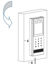
Put the device into the bracket and push it down, then insert Allen wrench into the bottom of the device, and turn the wrench 45-degree clockwise. After that, push down the device all the way, then turn the Allen wrench 90-degree counterclockwise.
