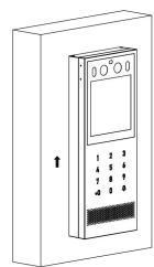
Push the device upward to check if the installation is complete. If the device still moves, please repeat the above steps.
