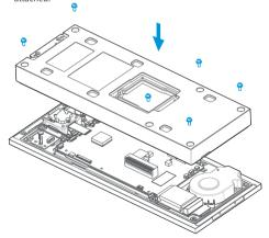
Put the rear cover to the device and tighten the cover using the six screws (M3x9)that are previously removed.
