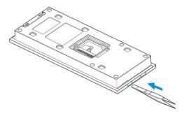
Push the card against the slot base using the back end of the tweezers until you hear a clattering sound when the SIM card will be pushed out.
