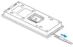
Take out the SIM card from the slot using the tweezers tips.
