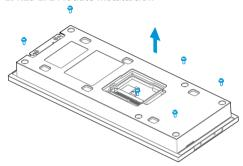
Remove the six screws (M3x8) on the device's rear cover using cross screwdriver and keep the screws.
