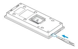
Insert the SIM card to the card slot at the bottom and push the card all the way in using the back end of the tweezers attached with the module until you hear a clattering sound.
