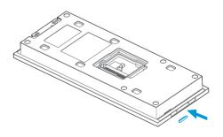
Plug the SIM card slot using the silicone plug attached.
