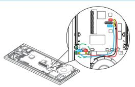
Connect the main RF cable and the div RF cable to the module as indicated in the dotted green circle. While the other ends of the two cables are already connected to the main-board.
