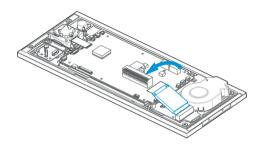
Insert the LTE module connecting fingers into the interface as indicated in the drawing and press down the other end of module to line up the left screw hole with the lower screw column.
