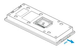
Remove the SIM card rubber plug at the bottom of the device.
