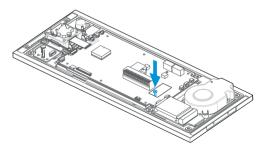
Lock the module on to the screw column of the device with the screws (M2x5).
