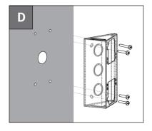
Tighten the four **ST4x20 crosshead screws** to the **plastic wall anchors** to fasten the **adjustable angle bracket**.
