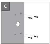
Insert four **plastic wall anchors** into four drilled holes.
