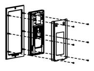
As shown in the picture, combine bracket, device, and plate together. Secure them by fixing six M3X8 crosshead screws.
