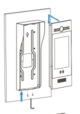
Install the device on the wall-mounting box , press down the device and make sure that the two hang holes on its top are fully hanged on to the two square hooks on the top of the box, then tighten the two countersunk machine screws (M3x6) underneath the device using the Allen wrench attached with the device.
