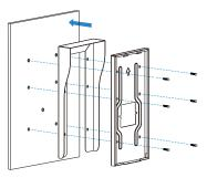
Combine the wall-mounting box with the rain cover and mark the six mounting hole positions on the wall. Drill the holes and insert the six plastic wall anchors into the holes according to regular device installation requirement. Then tighten the combined rain cover and the box securely on the wall using the six tapping screws (ST4x20).
