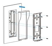
Install the embedded box on the wall according to its installation manual. Combine the flush-mounting bracket with the rain cover before tightenining them securely on the wall using the 6 screws(M4x10) attached with the device.
